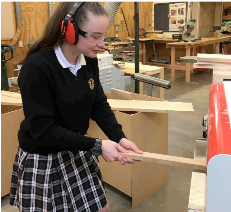
Using a thicknesser to ensure all seat planks are the same thickness.
