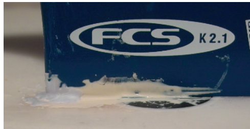
Surf board fin repaired with epoxy resin
