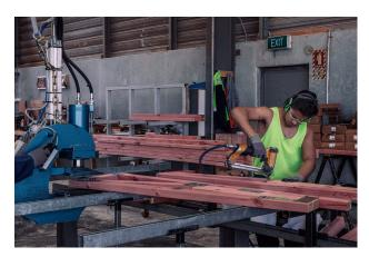
Frame and truss manufacturers make prenailed framing sections of walls and roofs.
