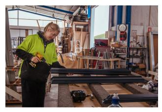
Sometimes called aluminium fabricators, architectural aluminium joiners machine and fabricate aluminium into joinery items. Most of their work is in creating aluminium framing for windows and doors but sometimes they need to create aluminium joinery for features, such as round windows, specified in the building plans.
