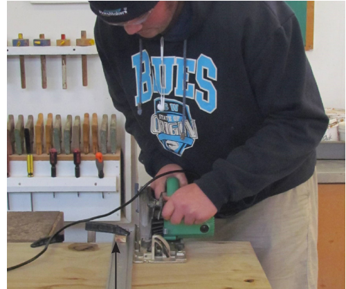
F clamps located at either end of the over-centre locking guide bar for extra security
