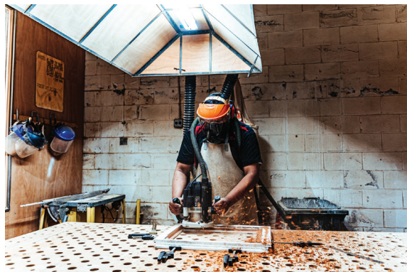
Rebating a timber window frame
