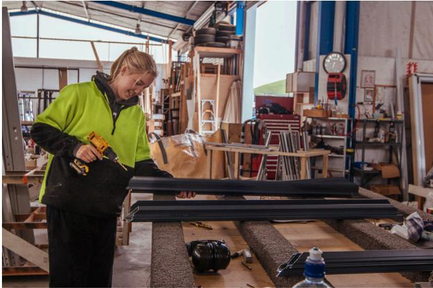
Sometimes called aluminium fabricators, architectural aluminium joiners machine and fabricate aluminium into joinery items. Most of their work is in creating aluminium framing for windows and doors but sometimes they need to create aluminium joinery for features, such as round windows, specified in the building plans.
