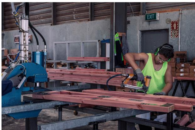
Frame and truss manufacturers make pre-nailed framing sections of walls and roofs.
